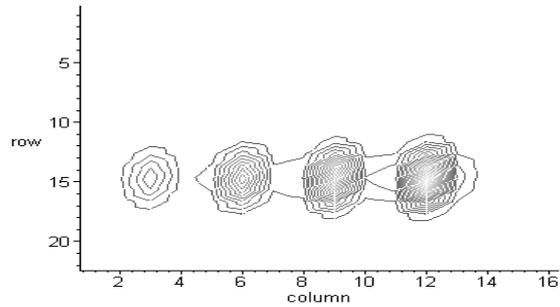
**Figure 7. Contour map of utility functions for multiple objects experiment. Column number indicates the distance from the robot. Each peak is the centre of red, blue, yellow and green object (from left to right).**
