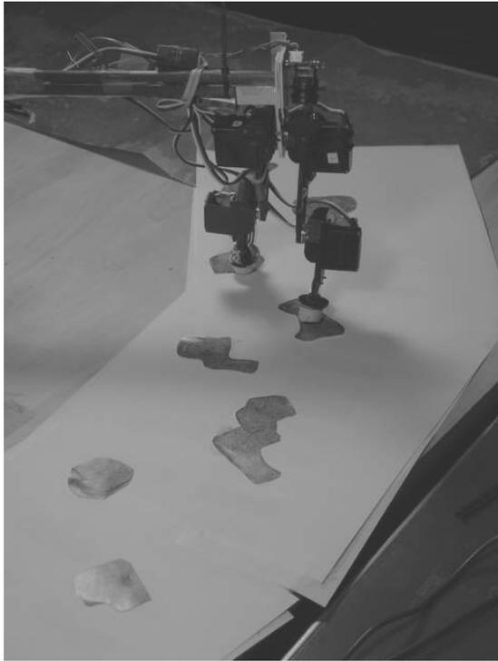
**Figure 1. Experimental setup.** A small (15cm) bipedal mechanism is shown. The textured regions represents areas of high walking utility, the white regions represent areas of low walking utility.
