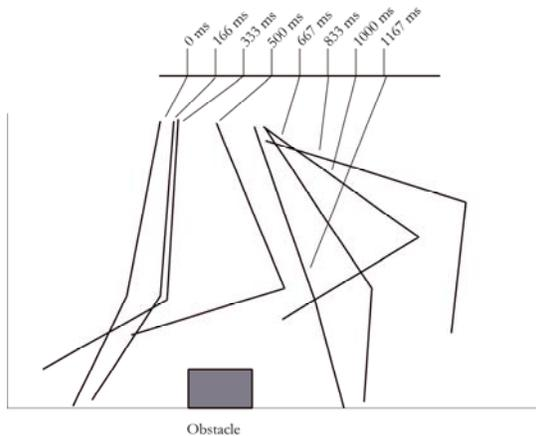
**Figure 3. From video data of the real robot while stepping over an obstacle. Kinematic diagram of the right leg of the robot stepping over an obstacle under automatic control of the learning algorithm here.**
