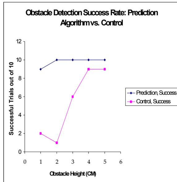
**Figure 2. Obstacle detection success rate.** The light gray line indicates success rate when no phase dependent prediction is used. As can be seen, objects must be about 4 cm or taller to be reliably detected. In contrast, the dark line shows the success rate with prediction. The results are much better, particularly for small feature size. See [1] for a full description of the experimental setup.
