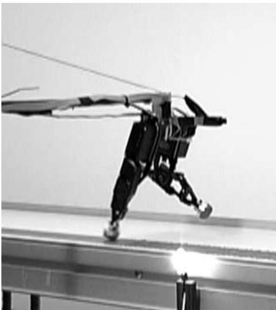
**Fig. 1.** RunningMan Biped on treadmill. Mechanism is about 14 cm tall. Hips are actuated. Knees are passive. The foot is a round pad
